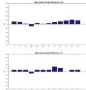
Figure 2: Absolute differences between Philips and CardioSecur in R-Peak amplitude.
