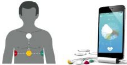
Figure 1: Electrode Placement and technical components of CardioSecur
